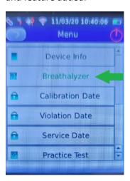
Once the feature is added, choose the Breathalyzer option from the second menu, as shown above, to provide a pre-test. The Pre-Test result will be displayed and stored on the unit but not reported to DMV/court. Be aware that a successful Pre-Test, even if the result is lower than the state fail point, will not allow you to start your vehicle. You will need to return to the main menu and proceed with a normal breath test to start your vehicle.
